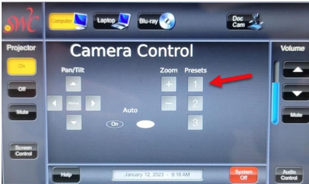
Pressing the “On” button will enable automatic tracking (Camera will follow the presenter). Auto tracking will be “Off” by default.
